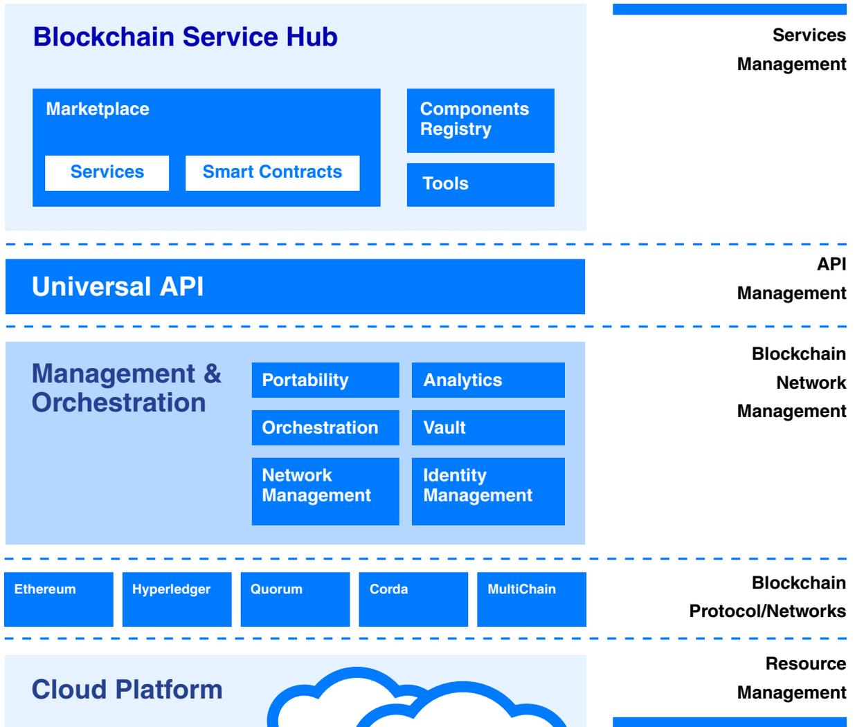
Basic Architecture of the Chainstack Platform
